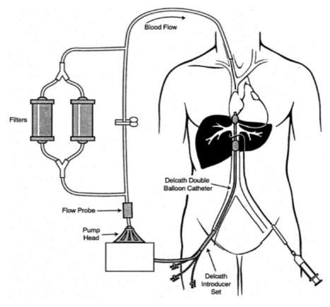
The Delcath PHP System kit includes the following disposable components manufactured for Delcath by third parties:
